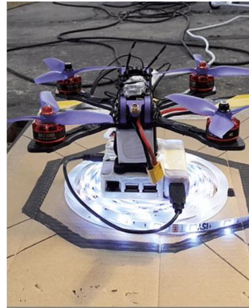
Inductive Charging via DroneHangar
